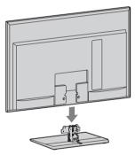
2 Fix the TV to the Table-Top Stand according to the arrow marks ★ that guide the screw holes using the supplied screws.
